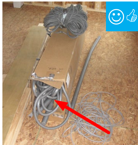
C. Backer-rod is a foam product available in various diameters that can be used to air seal openings around doors and windows.
